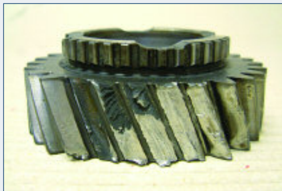
Shock loadings from can cause consequential damage.
