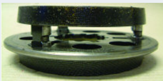
Synchro damage from oil leak.
