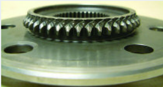
Consequential damage from synchro material failure.
