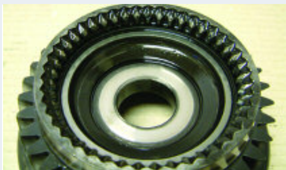
Consequential damage from synchro material failure.
