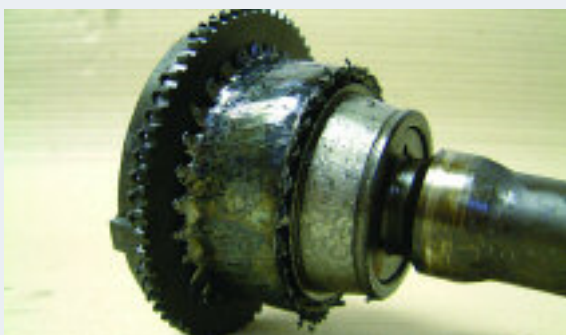
Low oil level damage.
